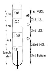
Fractioning of the density gradient after centrifugation. The density composition of the discontinuous gradient is indicated on the left. After centrifugation the VLDL are removed from the top of the gradient and the other fractions are collected through the base of the tube. The volumes of the fractions are indicated on the right of the figure.
